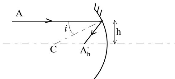
We can calculate in a similar way as for the refractive surface the position of the intersection point  $A'_h$  as a function of the height  $h$  of an incident ray originating at the object at infinity. We get:
