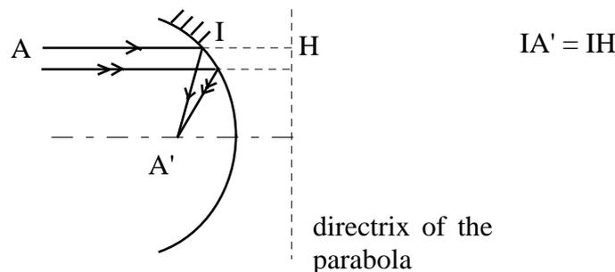
We should point out that this kind of mirror rapidly gives low quality images when the object moves away from the ideal focus. It is used for example to collimate the light beam of a high intensity source (we place the source at  $A'$  in order to get a parallel beam after reflection), to collect solar energy, and also very often in astronomy as the primary mirror.
