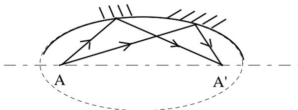
This kind of mirror is used for example to pump laser crystals such as Nd:YAG with a discharge lamp, the lamp being located at one of the foci of the ellipse and the laser crystal at the other (the section is elliptical, the system is invariant by translation in the perpendicular direction). If we want to increase the pump power by adding a second lamp, we then choose a
