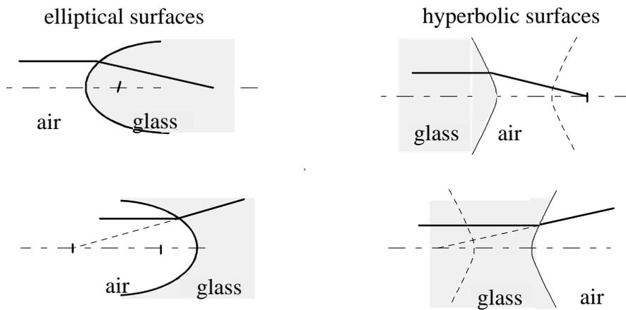
We will now see an example of use of these spherical refractive surfaces in condition of perfect stigmatism. Other combinations of refractive surfaces that form perfectly stigmatic lenses will be seen in chapter VII (§III.1).
