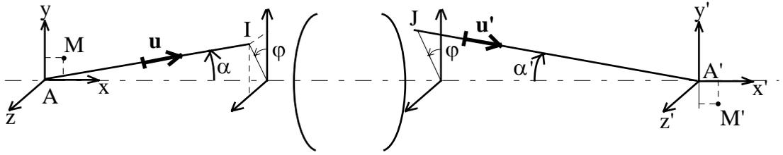
Since the system is perfectly stigmatic for  $A$  and  $A'$ , the optical path  $(AIA')$  is independent of  $I$ . The condition  $(MIM')$  independent of  $I$  can thus be written as:
