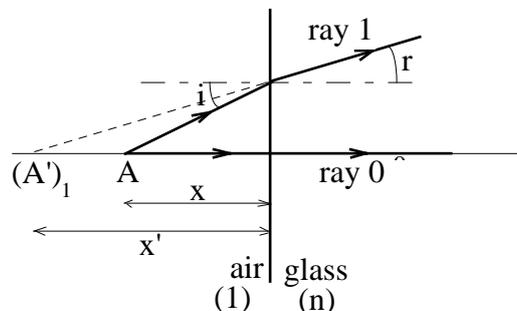
Applying Snell-Descartes' law for refraction, we can calculate the position  $x'$  of the intersection  $(A')_1$  of rays 0 and 1:
