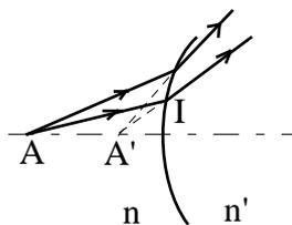
To calculate the optical path, virtual paths are counted with a negative sign. For example in the case of a surface between two media with indices  $n$  and  $n'$  (see figure above), the optical path from A to A' is given by:
