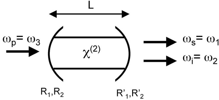
FIG. 1 – *Optical parametric oscillator*
