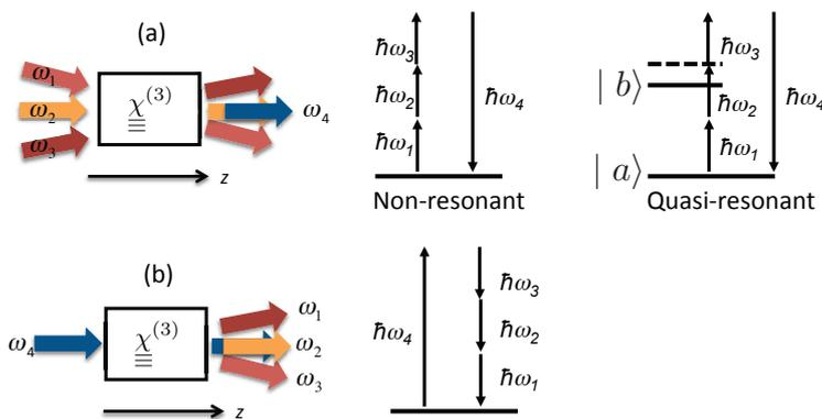
**Fig. 4.1.** Four Wave Mixing schemes. (a) The interaction between three waves at  $\omega_1$ ,  $\omega_2$  and  $\omega_3$  generate a fourth wave at  $\omega_4 = \omega_1 + \omega_2 + \omega_3$ . (b) One single intense pump beam at  $\omega_4$  can generate 3 waves at  $\omega_1$ ,  $\omega_2$  and  $\omega_3$ .
