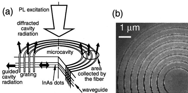
FIG. 2. (a) Schematic of the microcavity with circular trenches and measurement of resonances through localized detection of air-diffracted PL; (b) micrograph of a typical disk.
