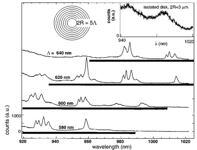
FIG. 3. Raw spectra of light collected selectively on the grating area of disks with pitches  $\Lambda = 580, 600, 620,$  and  $640 \text{ nm}$ , and diameters  $2R = 5\Lambda$ , with a vertical shift for clarity; stop bands of the grating are represented as dark bars below each curve. Inset: spectrum of stray light from an isolated disk of diameter  $2R = 3 \mu\text{m}$  showing only smooth features.
