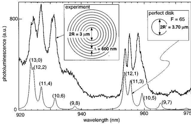
FIG. 4. Experimental data (upper curve) and simple disk model (bottom curve) for the  $R=3\ \mu\text{m}$ ,  $\Lambda=600\ \text{nm}$  structure. The finesse has been adjusted to 65 and the diameter to  $2R'=3.70\ \mu\text{m}$ . Numbers in parentheses are the mode numbers  $(m,n)$ .
