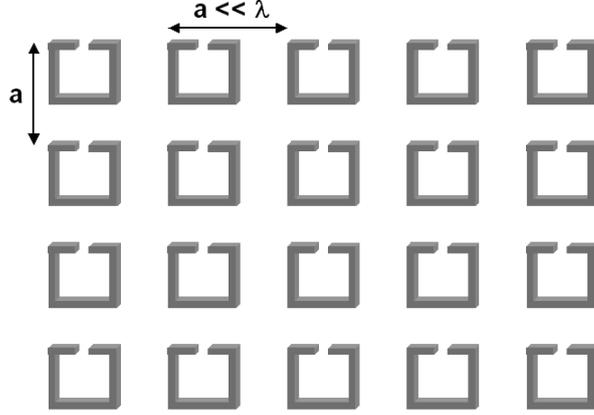
Metamaterial made of a cubic array of metallic split-ring resonators (SRRs).
