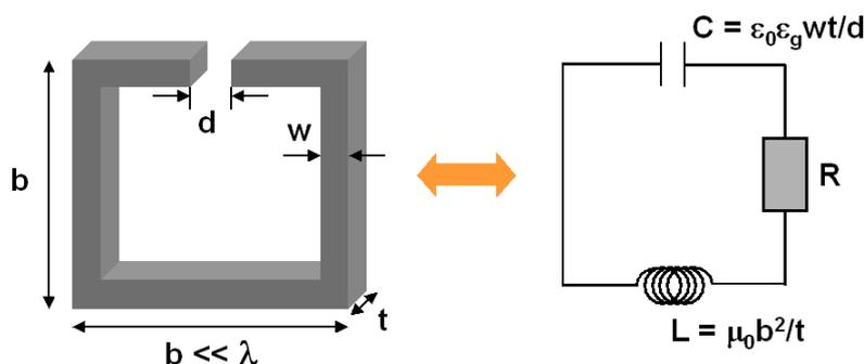
Analogy between a split metallic ring with a size much smaller than the wavelength and a RLC circuit.
