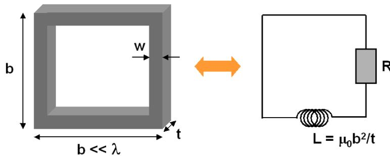
Analogy between a closed metallic ring with a size much smaller than the wavelength and a RL circuit.
