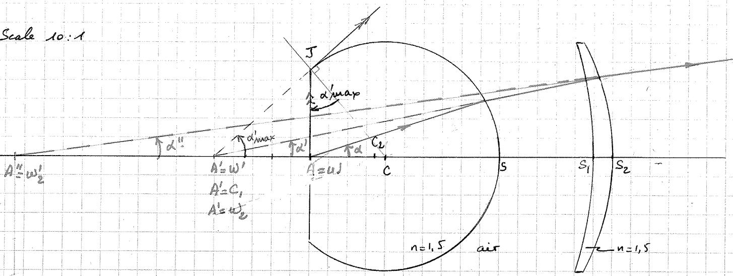
a) Object A at object Weierstrass point of the glass "sphere":  $\overline{CA} = \frac{1}{n} \overline{SC} = \frac{2}{3} R$
